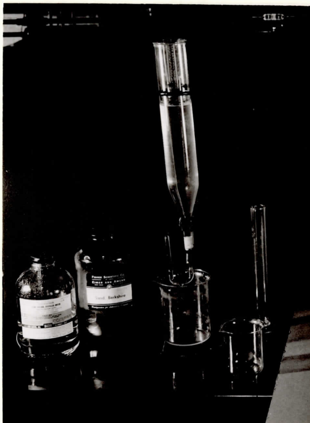
Figure 16. SEDGWICK-RAFTER SAND FILTER
